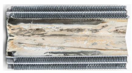
The images show how deposits can form inside your radiator's cooling tubes, blocking flow and preventing optimal heat transfer. By using a quality nitrite-free coolant like Cool-Gard II, you eliminate this kind of deposits formation, allowing full heat-transfer capability and efficiency.
